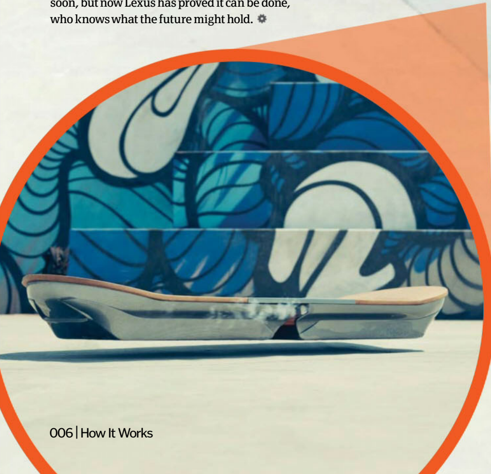
Unlike its movie counterpart, the hoverboard can also work over water, provided that there is a magnetic track underneath
