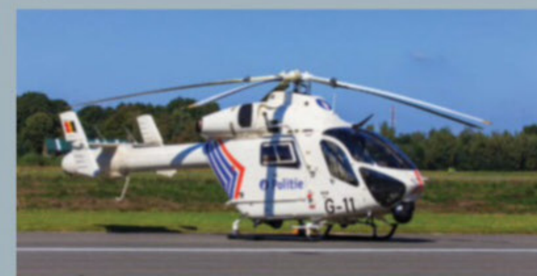
This Belgian police helicopter features the innovative no-tail rotor (NOTAR) system
