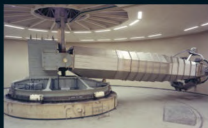
This centrifuge is designed to test the effects of linear acceleration on visual function in space
