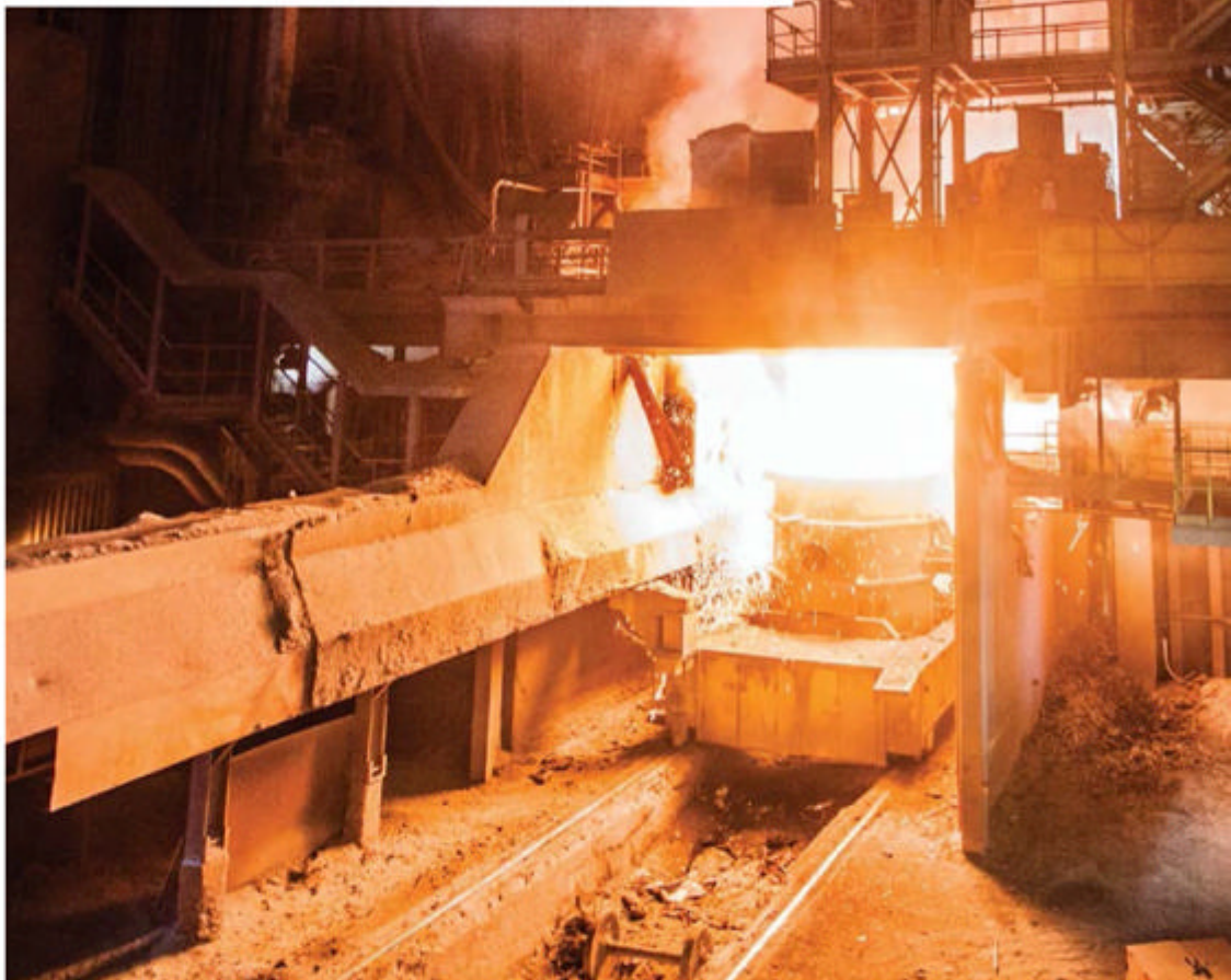
The tapping of the molten steel is an incredible sight. Extra elements like silicon are added at this stage to create the right grade of steel
