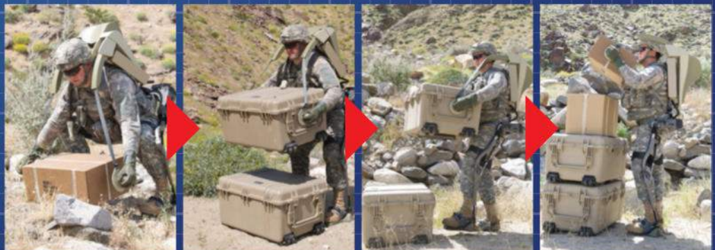
The HULC exoskeleton enables soldiers to comfortably carry up to 91kg (201lb)
