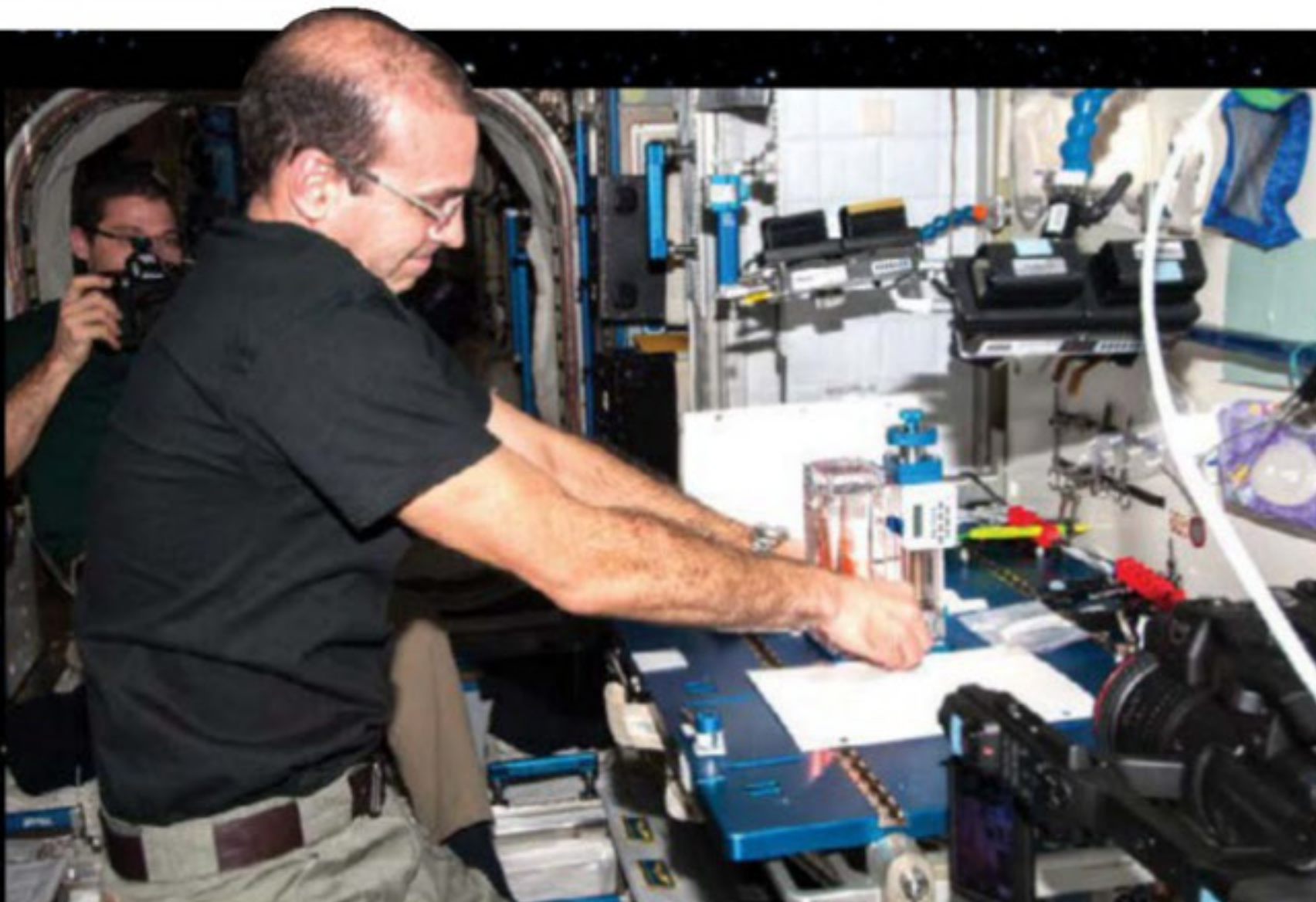
ABOVE Rick Mastracchio investigating how fluids act in microgravity on the ISS. The results of this experiment could benefit future liquid delivery and containment on the station and other spacecraft
