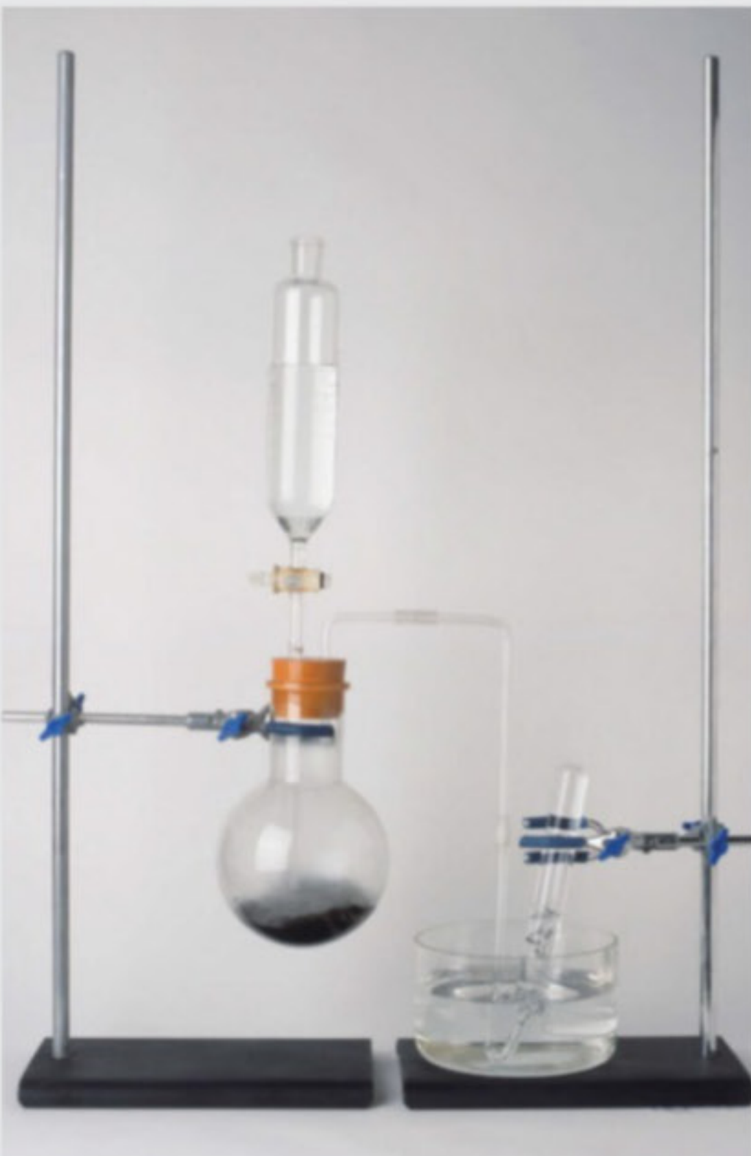
ABOVE Catalysts can aid the production of oxygen by decomposing hydrogen peroxide
