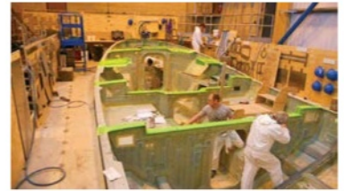
These images show the process of building a Shannon lifeboat, from setting the hull to adding the cabin
